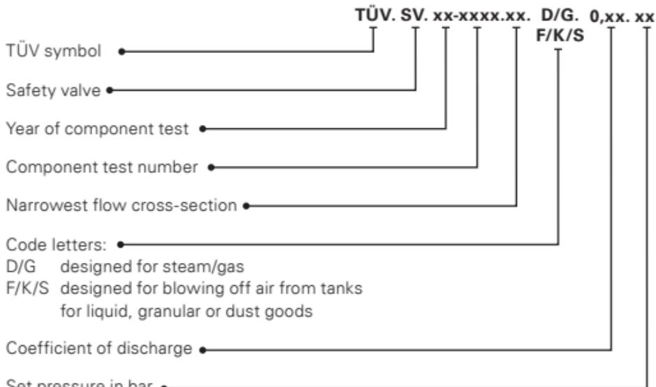
We check the safety valves for pressure resistance and tightness, adjust the requested set pressure and seal them.
